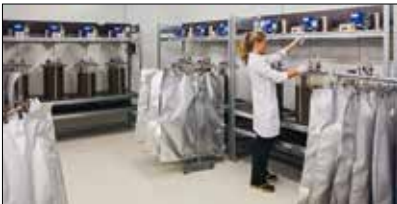
Continuous biogas fermenters
